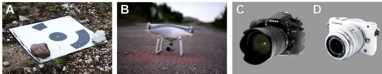
Fig. I. The selected equipment for the photogrammetry method applied at Dingwall; A – largest portable PCV board 42×45.5 cm used as a control point; B – Unmanned Aerial Vehicle DJI Phantom 4 Advanced; C – Nikon D7100; D – Olympus E-PL 6 Lite.
