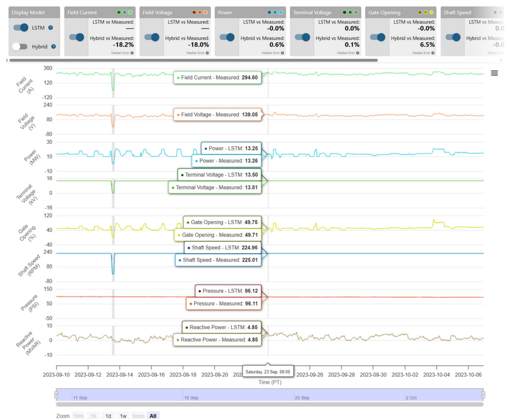
Figure 9. Screenshot from the “online” mode viewer on the DT data portal showing the LSTM models’ outputs for the U12 unit. The depicted period covers 10 September 2023, through 6 October 2023.
