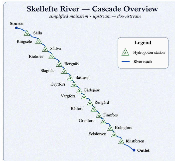
Figure 1. Schematic representation of hydropower stations along the Skellefte River based on the stations listed in Table 1. The figure is illustrative and not a georeferenced map.
