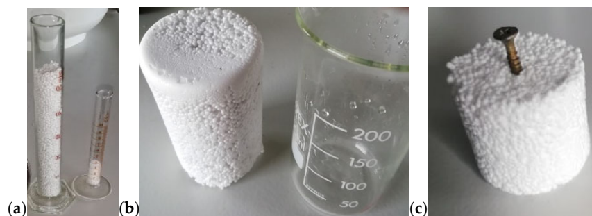
Figure 14. Volume occupied by EPS beads (a) before and (b,c) after the MW-assisted heating.
