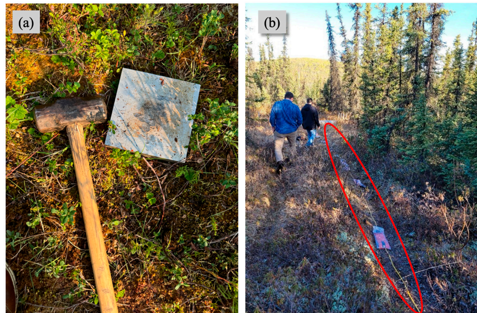
Figure 3. (a) Photograph of sledgehammer and metal plate utilized for active source impacts. (b) Photograph of the May 2025 weighted portion of fiber optic cable (circled in red) [32].
