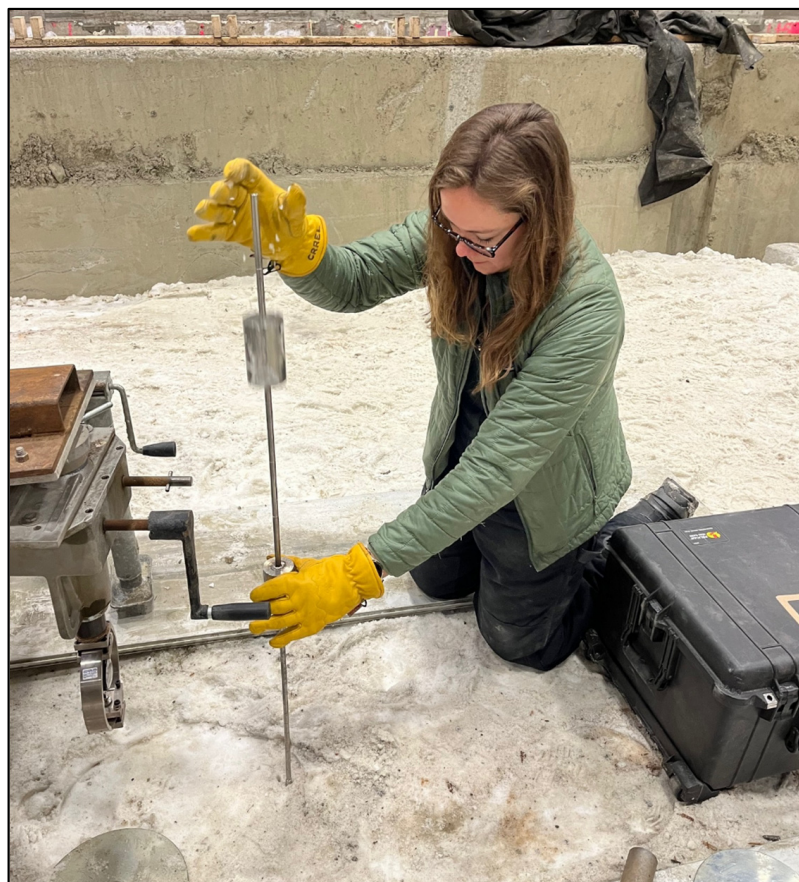
Figure 3. A researcher performing the RSP method for measuring the strength of the compacted snow pavement test section prior to the corresponding CBR measurement.
