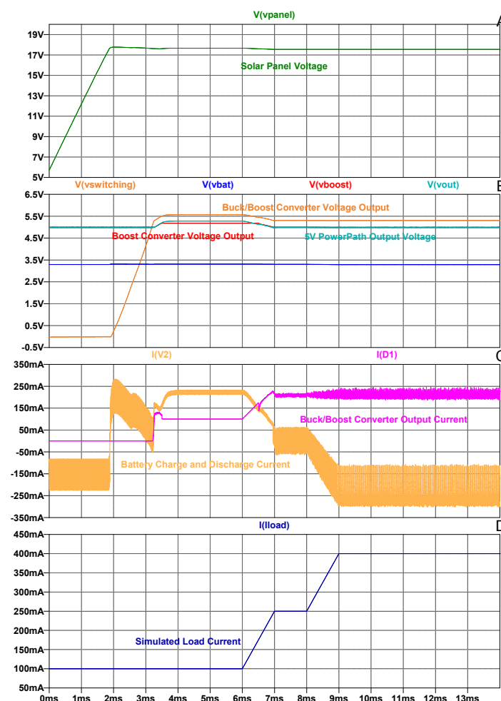
Figure 15. Simulated transient response of the PowerPath circuit under partial irradiance with a stepwise increasing load. (A) Solar panel voltage. (B) Buck/Boost converter output ( V_{boost} , orange), Boost converter output ( V_{boost} , red), 5 V PowerPath output ( V_{out} , cyan), and battery voltage ( V_{bat} , blue); the output rail remains regulated throughout the commutation event. (C) Buck/Boost converter output current ( I_{D1} , magenta) and battery current ( I_{V2} , orange); the battery transitions from charging to active discharging as the load demand exceeds the solar-derived supply. (D) Simulated load current profile, ramping from 100 mA to 400 mA.
