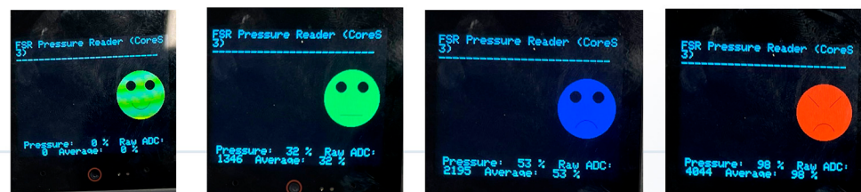
Figure 1. Pressure-Dependent Emotional State Transition and Facial Expression Mapping. The figure illustrates the relationship between normalized pressure input values (P) and the corresponding emotional states generated by the proposed affective sensing system. As the applied pressure increases from left to right, the system transitions through multiple emotional response regions, each associated with different facial expressions, visual feedback patterns, and optional audio responses. The normalized pressure signal is continuously processed and mapped to predefined emotional states using threshold-based classification combined with linear interpolation between adjacent states. This interpolation enables smooth transitions in facial parameters, including mouth curvature, eye shape, and eyebrow angle, rather than abrupt switching between discrete expressions. The figure additionally summarizes how increasing pressure intensity influences the perceived emotional response and interaction feedback presented on the embedded LCD display.
