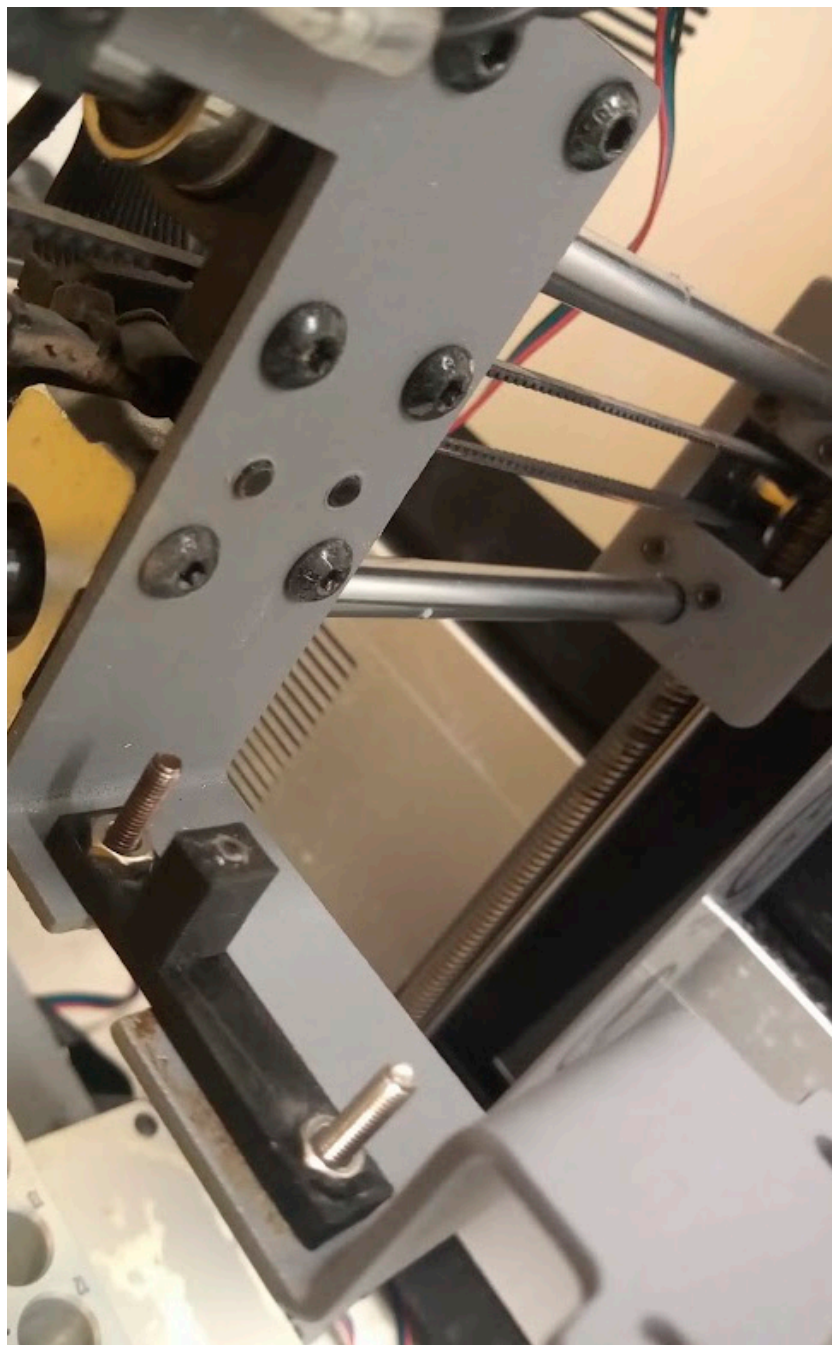
Figure 2. Custom 3D-printed tube holder attached to the extruder support on the 3D printer.
