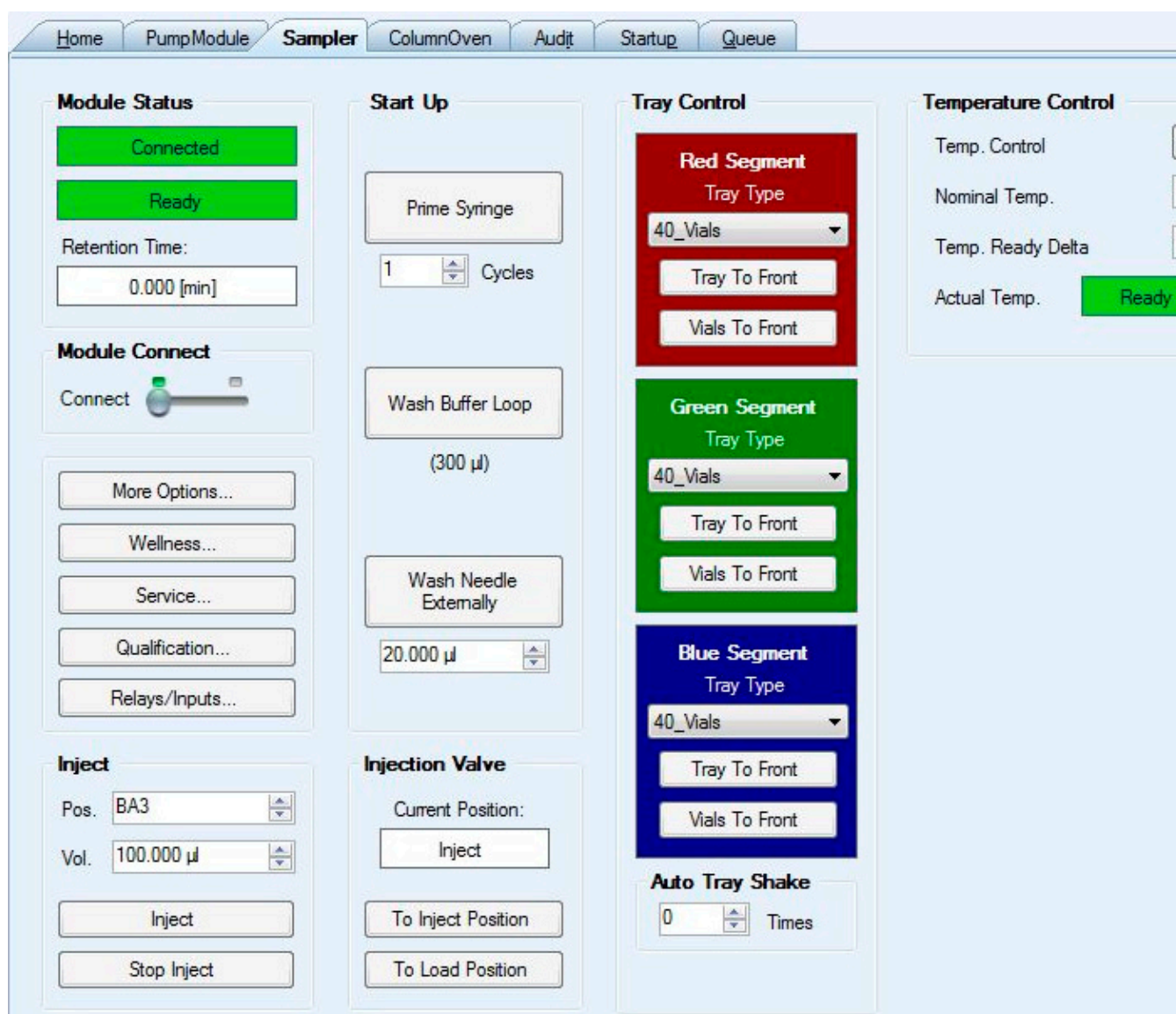
Figure 19. Chromeleon interface for autosampler control. Commands were sent to the “Pos.” input box, and to the “Inject” button.
