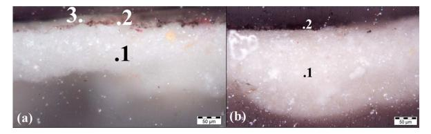
**Figure 11.** Microphotographs of sample cross sections: (a) ORM 12: lime from the plaster (1), redbrownish (probably degraded pigment) colour layer a fresco (2), white colour layer a fresco (3), St. Martin scene, north wall. (b) ORM 10: lime from the plaster (1), darkened colour layer (2), decoration bordure under the four female saints. Triumphal wall of the nave, St. Jacob's church, Ormož, Slovenia.
