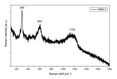
**Figure 10.** Raman spectrum of the sample ORM 3 identifying tenorite by its characteristic Raman vibrations at 300 and 600 cm<sup>-1</sup>. Sample from the first female saint's coat, lower pictorial band, triumphal wall of the nave, St. Jacob's church, Ormož, Slovenia.
