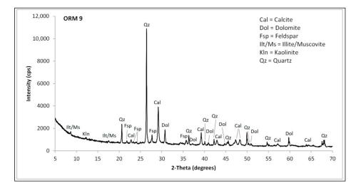
**Figure 4.** XRD pattern reveals a plaster made with a higher amount of aggregate and less binder, with some impurities. Sample from the pinkish soil, Adoration of the Magi, triumphal wall of the nave, St. Jacob's church, Ormož, Slovenia.
