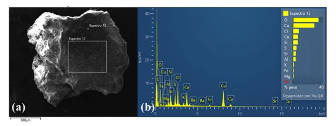
**Figure 8.** Raw sample ORM 11. (a) SEM image with marked point (13) and area (12) of EDS analysis; (b) EDS spectrum of the point analysis indicating the presence of green earth (Mg, Al, Si, S, K, Fe) and malachite (Cu) degraded to (para)atacamite (Cu, Cl). Sample from the green background, north wall of the nave, St. Jacob's church, Ormož, Slovenia.
