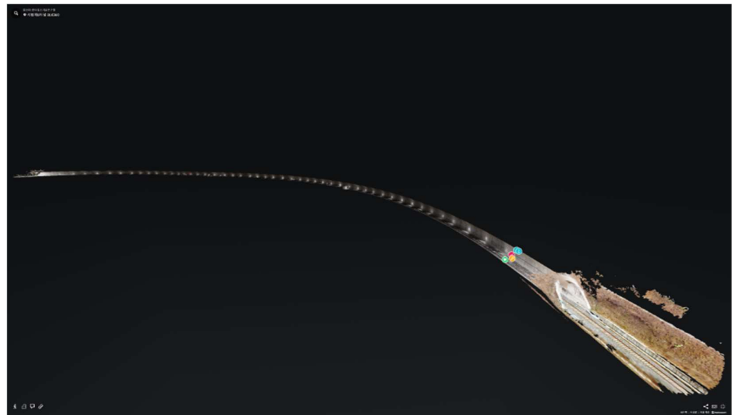
Figure 5. 3D model of test tunnel 6 using Matterport Cloud (example).
