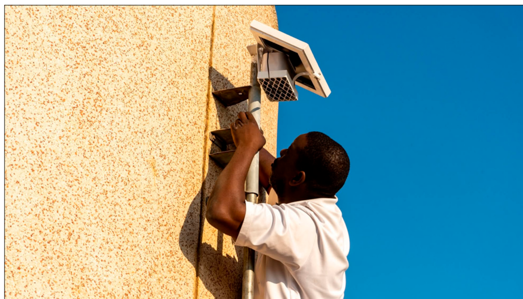
Figure 2. Setting up an air quality monitor at one of the sites.
