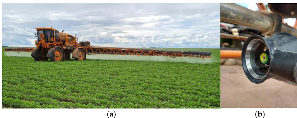
**Figure 1.** Self-propelled sprayer (a) and electrostatic nozzle body (b) used in applications.
