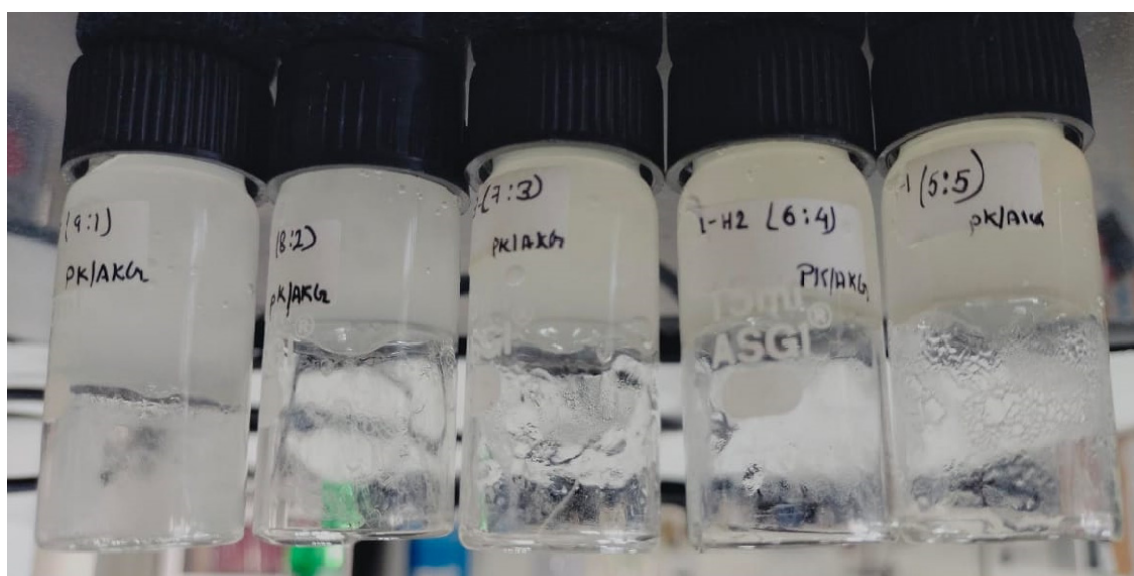
Figure 1. Visual observation of blank hydrogel with different PVA:CS ratios.
