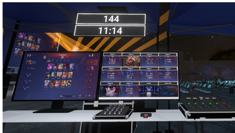
Figure 4. Broadcast switching and monitoring interface in the VR-based training environment, displaying multiple live video feeds, scene selection panels, production status information, and controls for managing broadcast transitions during esports events.
