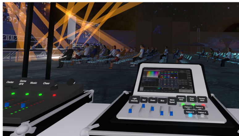
Figure 3. Virtual lighting control interface in the VR-based training environment, showing lighting color selection, intensity adjustment controls, preset lighting functions, and a real-time preview of stage lighting effects within the simulated esports venue.
