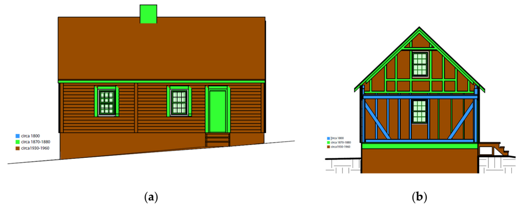
Figure 14. Color-coded Revit model: (a) North elevation; (b) section looking West.
