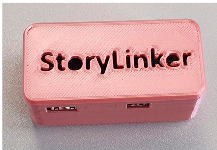
Figure 7. StoryLinker Dongle housed in a custom 3D-printed enclosure.
