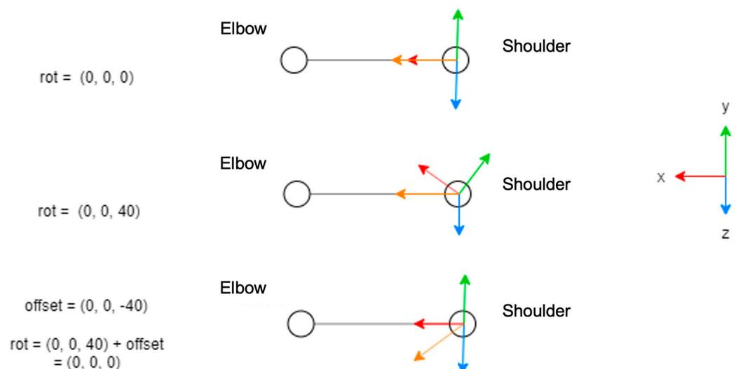
**Figure 6.** Rotation axis correction.
