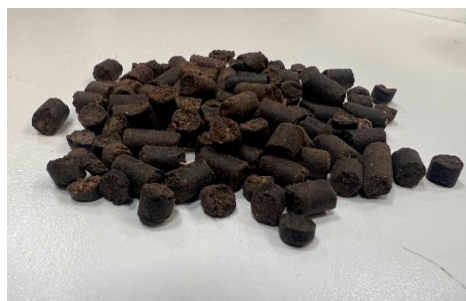
Figure 1. Dried olive pomace in the form of pellets was used in this study.
