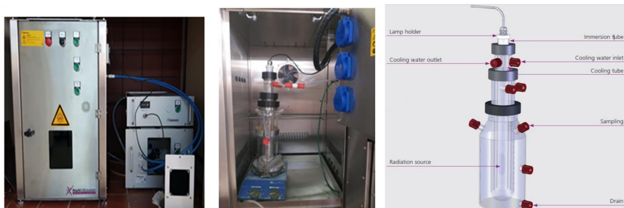
Figure 2. Photoreactor set up by Peschl Ultraviolet GmbH—Mainz, Germany; radiation protection cabinet; power supply and cooling unit ( left ); photoreactor vessel ( center ); vessel parts ( right ).
