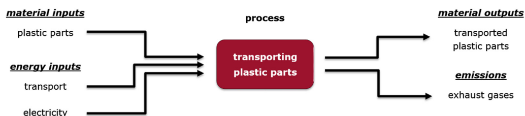
Figure 3. Inputs and outputs of the process module: "transporting plastic parts".
