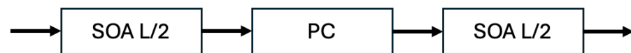
Figure 17. Schematic of the polarization-independent SOA. L is the length of the SOA. If the original polarization state is required, an extra PC can be added before the first SOA section or after the second SOA section.
