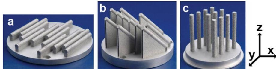
**Figure 13.** Static-tensile specimens built in different directions: (a) 0°, (b) 45°, and (c) 90°. Reprinted with permission from Ref. [15]. Copyright 2012 Elsevier.
