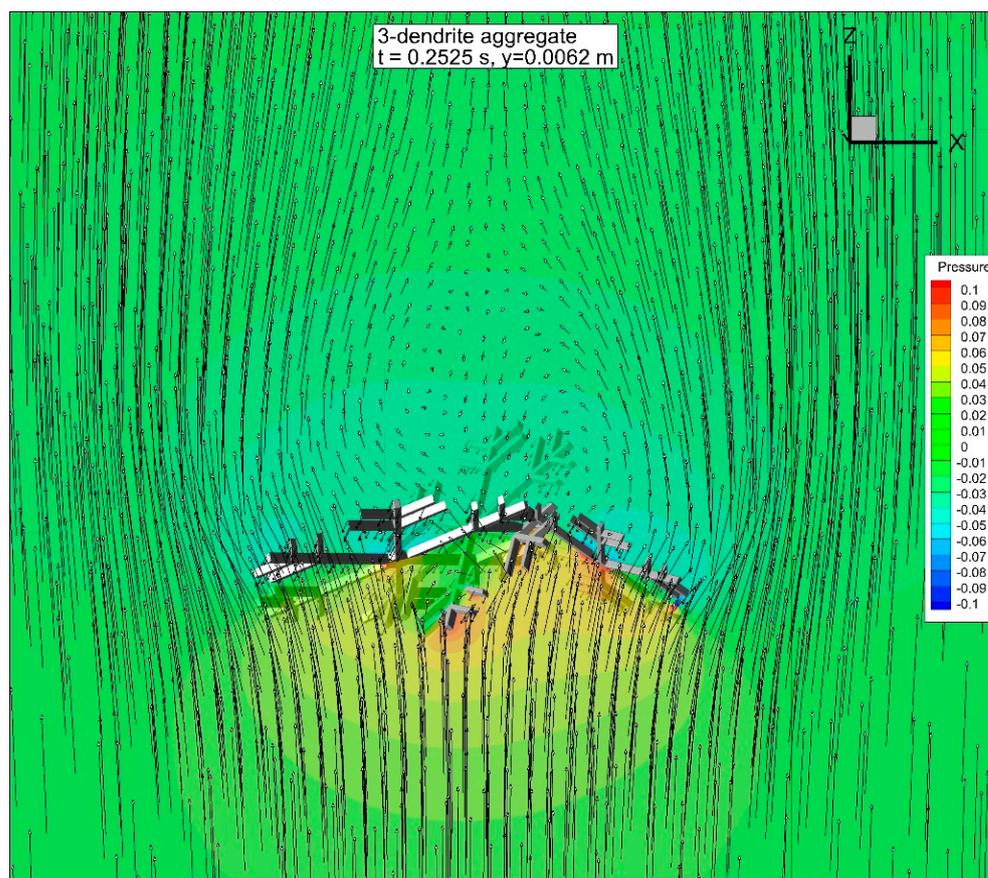
**Figure 19.** The velocity (arrows) and pressure (color) distributions around a falling snow aggregate consisting of 3 individual dendrites freely falling in air.
