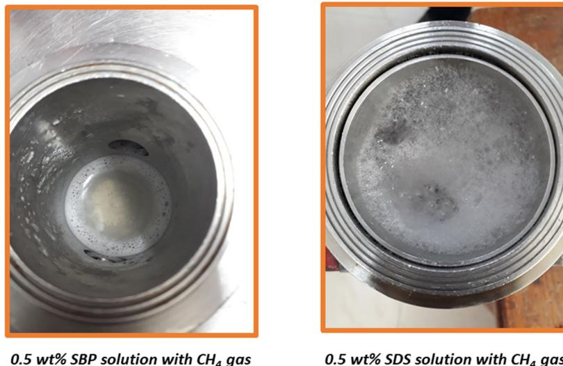
**Figure 5.** The figure shows the photographs of SBP and SDS solutions after the methane hydrate dissociation. The SDS system is where foaming is most frequently seen.
