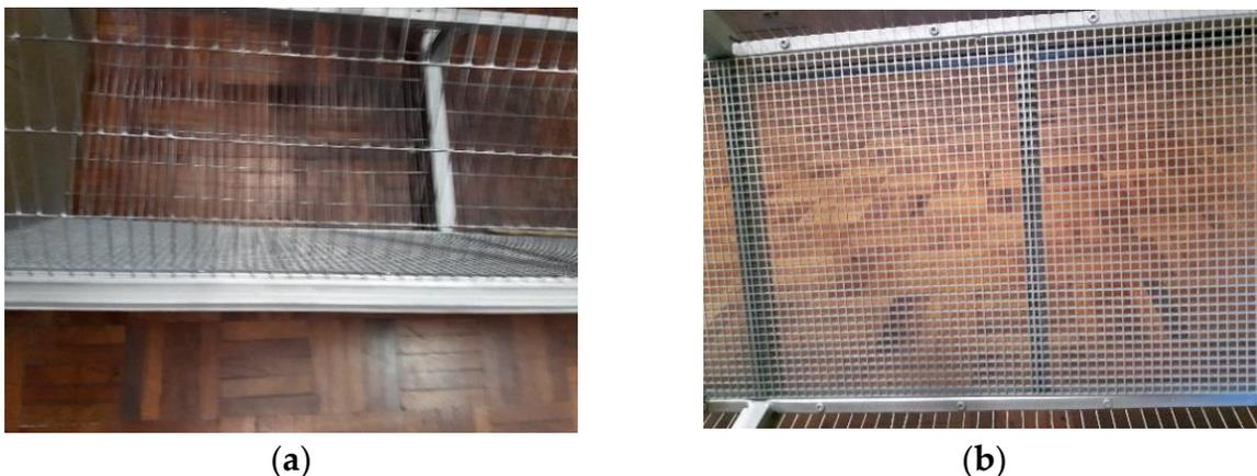
**Figure 4.** The model's: (a) deck beam and guard mesh, and (b) deck mesh.
