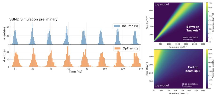
**Figure 5.** The timing structure of the BNB via light production: the light reconstruction is able to resolve the neutrino “bucket” structure of the beam spill (left). A preliminary estimate of different accessible areas of heavy neutral lepton phase space by SBND (right).
