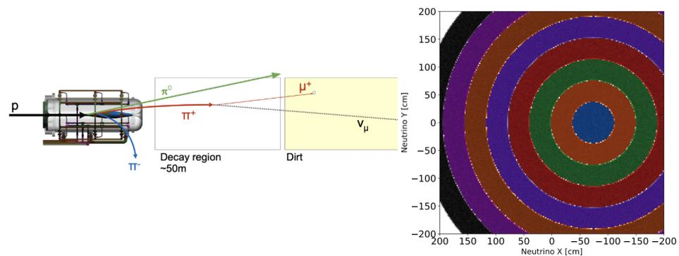
**Figure 3.** A schematic of the Booster Neutrino Beam showing charged and neutral meson production (left). Different off-axis angles (ranging from 0 to 1.8 degrees) for obtaining different neutrino energy spectra in SBND PRISM (right).
