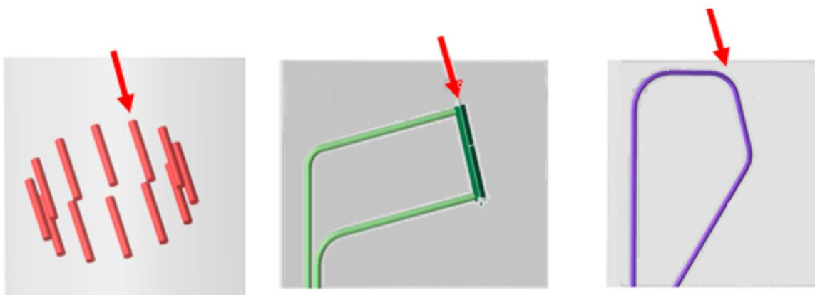
**Figure 1.** Three target design options. **(Left)**—rotating elements target; **(Center)**—fixed granular target with gas cooling; **(Right)**—conveyor-type target. The incoming beam direction is indicated by the red arrows.
