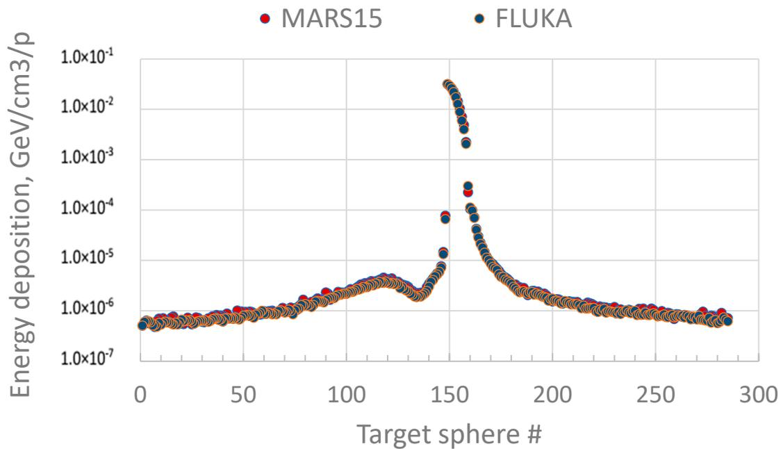
**Figure 3.** Energy deposition in W spheres as simulated with MARS15 and FLUKA. Target sphere # refers to the target sphere sequential number.
