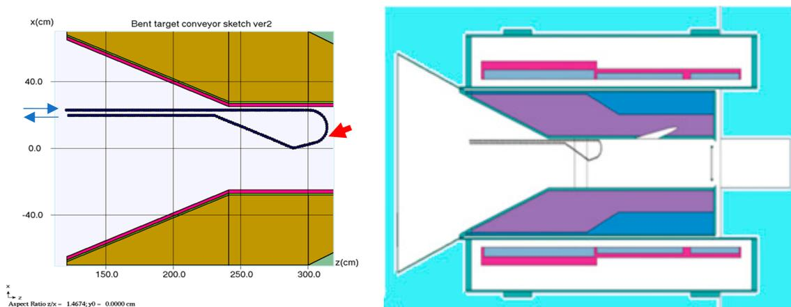
**Figure 2.** Simulation models of the W conveyor target within the HRS of the production solenoid. Red arrow indicates path of incident proton beam. (Left): MARS15. (Right): FLUKA.
