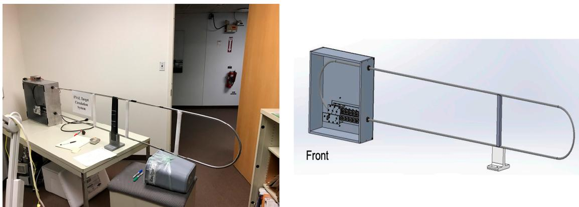
**Figure 5.** The first prototype of the conveyor target. (Left): as constructed. (Right): a CAD model used in the fabrication.
