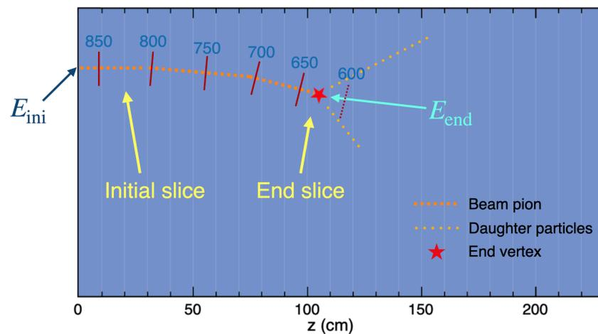
**Figure 1.** Demonstration of the energy slicing method. In this example,  $E_{ini} = 866$  MeV,  $E_{end} = 627$  MeV.
