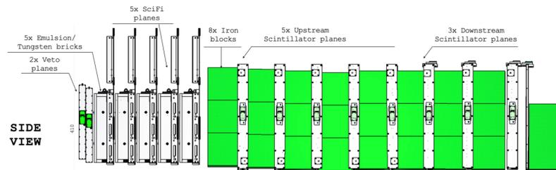
Figure 1. Layout of the SND@LHC experiment.
