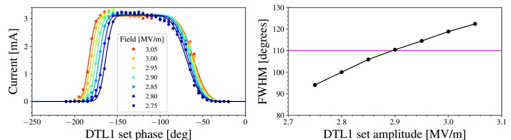
**Figure 3.** **Left:** DTL1 transmission vs. phase. **Right:** FWHM vs. amplitude. The model predicts a 110 degrees FWHM for the design 3.05 MV/m amplitude, indicating the set field being off by  $-5\%$ .
