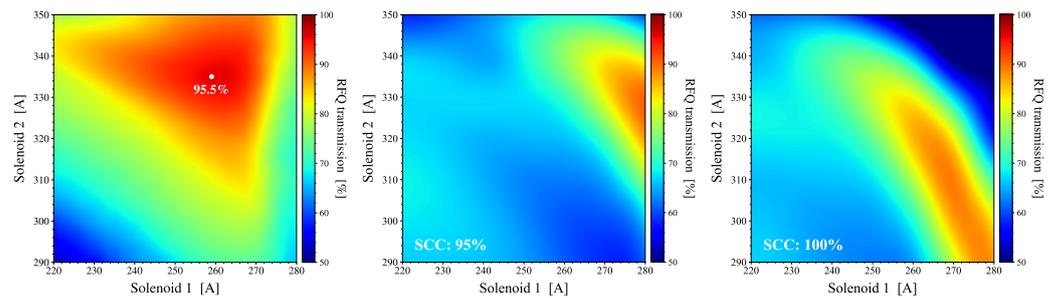
**Figure 2.** RFQ transmission vs. LEBT solenoids. **Left:** Measurement. **Middle:** simulations with a 95% SCC. **Right:** Simulation with 100% SCC.
