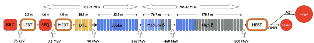
**Figure 1.** ESS linac schematic layout during the initial 2 MW Ops. The segments in the DTL and SC sections denote DTL tanks or cryomodules. The cryomodules in gray will not be powered during the initial Ops, making the beam energy and power 800 MeV and 2 MW for each.
