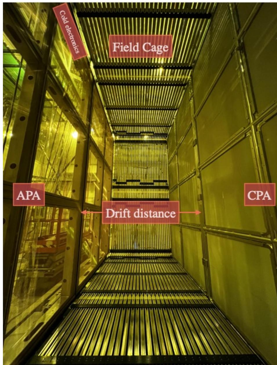
**Figure 3.** Picture of the assembled TPC showing the left-hand-side drift volume, with the main components labeled.
