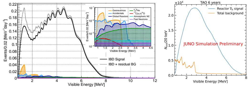
**Figure 1.** Left: Visible energy spectrum expected in JUNO detector as measured with (grey) and without (black) backgrounds. The inset shows the spectra of the expected backgrounds in log scale. Right: Visible energy spectra of reactor  $\bar{\nu}_e$  signal (blue) and total backgrounds (orange).
