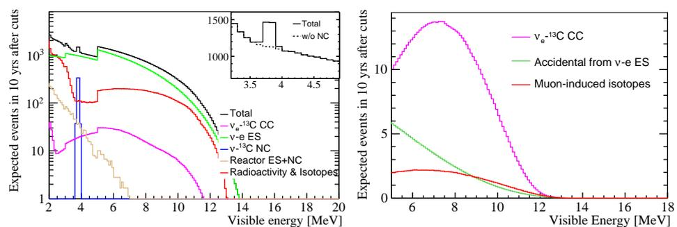
**Figure 4.** **Left:** Expected visible energy spectra of all single event sources for 10 years of data taking. The upper right insert plot is illustrated for the energy range between 3 and 5 MeV in the linear scale. **Right:** Expected prompt visible energy spectra of the CC signal and backgrounds after the optimized cuts for 10 years of running.
