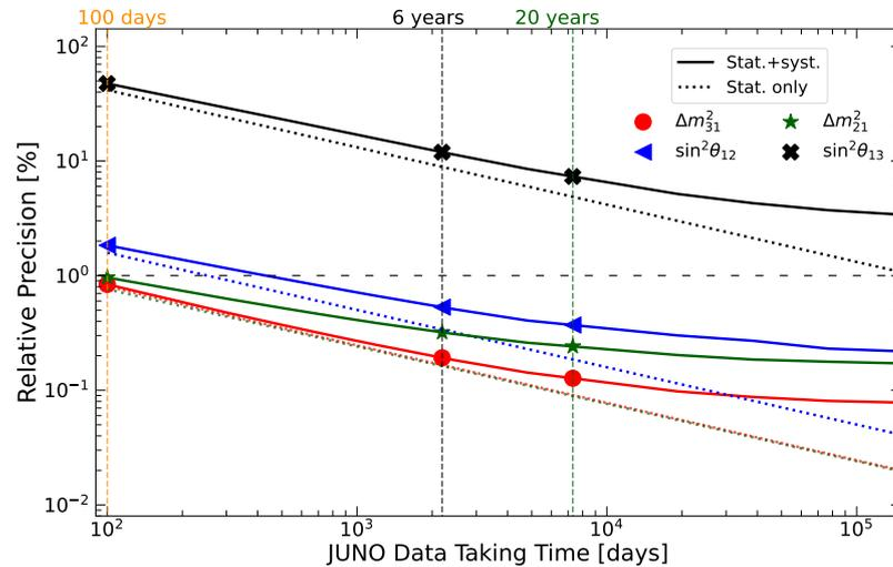
**Figure 3.** Relative precision sensitivity of the oscillation parameters as a function of JUNO data-taking time. The markers and vertical lines stand for 100 days, 6 years, and 20 years of data taking. The green and red dotted lines are on top of each other since the statistical-only precision is essentially identical for the  $\Delta m^2_{31}$  and  $\Delta m^2_{21}$  parameters.
