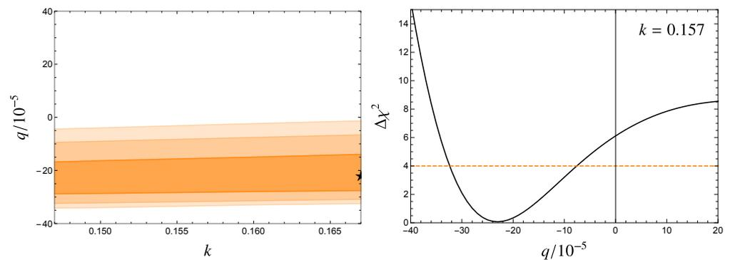
**Figure 1.** Left panel: The  $1\sigma$ , 90% CL, and  $2\sigma$  allowed regions in the  $(k, q)$  plane for the modified quenching factor model. The best fit point is marked by a star. Right panel:  $\Delta\chi^2 \equiv \chi^2(q) - \chi_{\text{min}}^2$  for a fixed  $k = 0.157$  [18].
