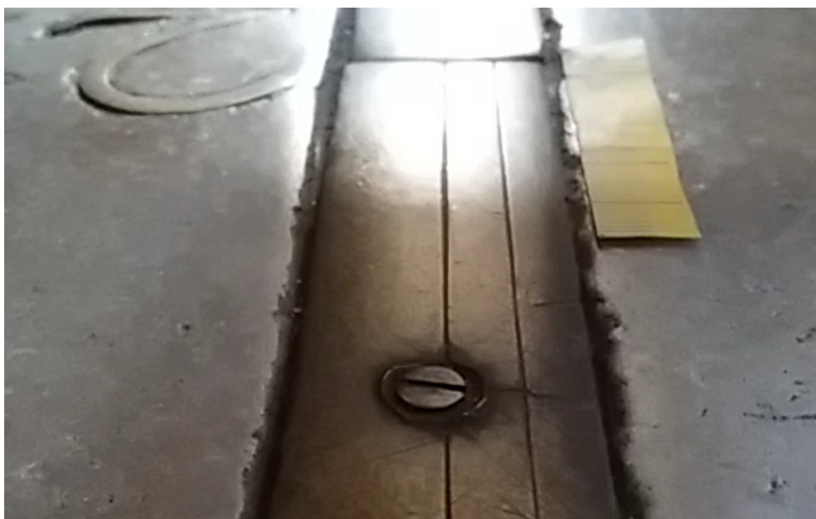
Figure 3. The southern limb of the Sun over 220 mark of the meridian line on 21 December 2020. The reddish penumbra is 5-mm thick, and the limb is darkened. On the right side, a paper meter with cm and mm marks is visible.
