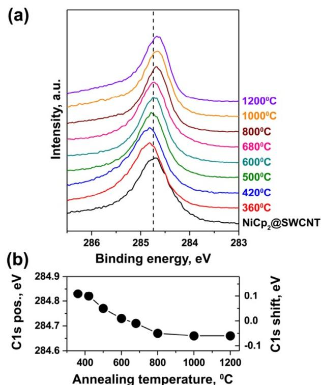
**Figure 3.** (a) The dependence of the electronic properties of nickelocene–filled SWCNTs on annealing temperature. (b) The plot of C 1s XPS position against annealing temperature. Copyright 2021 by the author. Licensee MDPI, Basel, Switzerland. This article is an open-access article distributed under the terms and conditions of the Creative Commons Attribution (CC BY) license [18].
