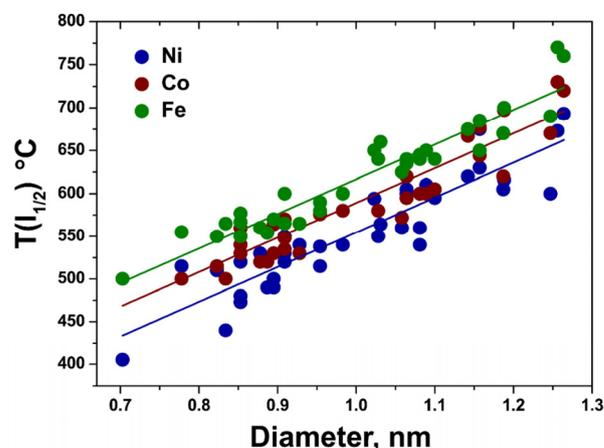
**Figure 2.** The growth temperature of nickelocene, cobaltocene, and ferrocene-filled SWCNTs was plotted versus the inner tube diameter. Copyright 2021 by the authors. Licensee MDPI, Basel, Switzerland. This article is an open-access article distributed under the terms and conditions of the Creative Commons Attribution (CC BY) license [16].
