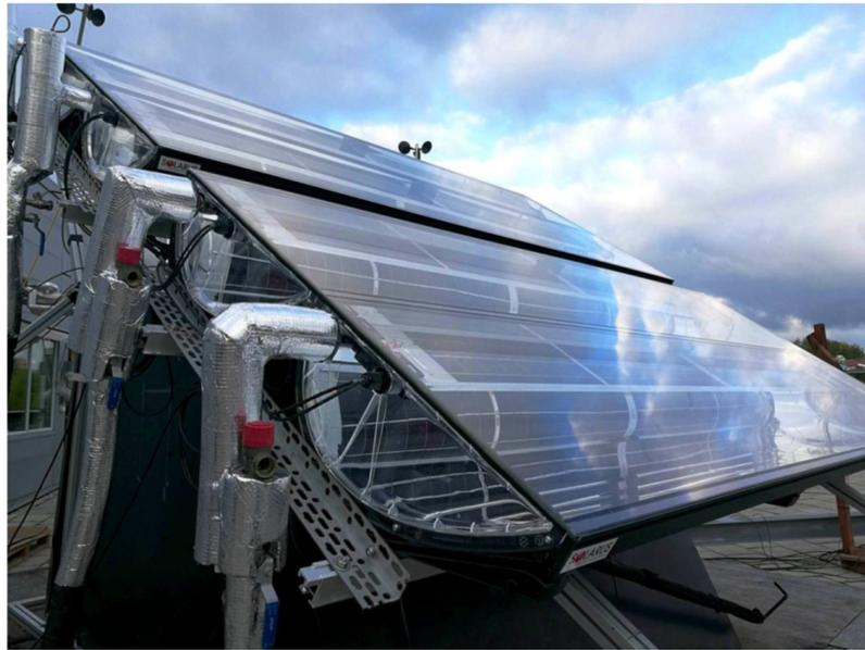
**Figure 5.** Rooftop collector mounting stand.
