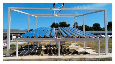
**Figure 2.** View of the prototype of LFC installed at the Plataforma Solar de Almería (Spain) during one of the tests to measure the flux of concentrated solar radiation in the focal plane.
