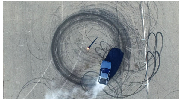
Figure 4. The circle drift scenario of a real car named MARTY [8]. The dark tire tracks on the ground clearly show the circular trajectory maintained during the drift.
