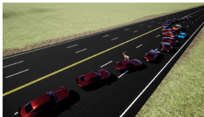
Figure 8. Drift maneuver used for collision avoidance [20]. The simulation demonstrates how a vehicle can utilize a controlled sideslip to navigate around an obstacle when conventional steering is insufficient.
