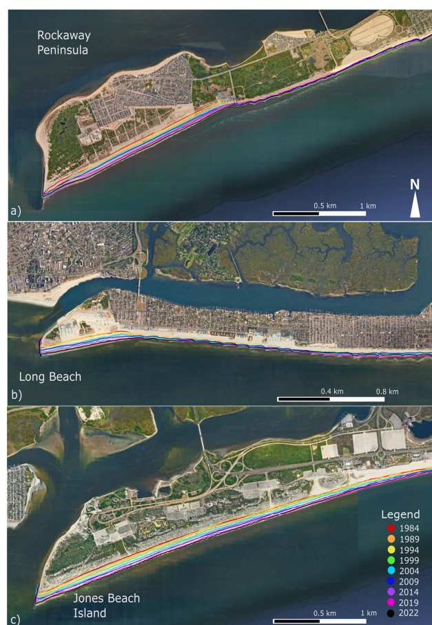
Figure 6. Western ends of each site showing the overall accretion using QGIS. See legend for color corresponding dates. The first continuous shoreline for each respective year was used for the visualization. (a) Rockaway Peninsula, (b) Long Beach, (c) Jones Beach Island. Images are from Google Earth within QGIS.
