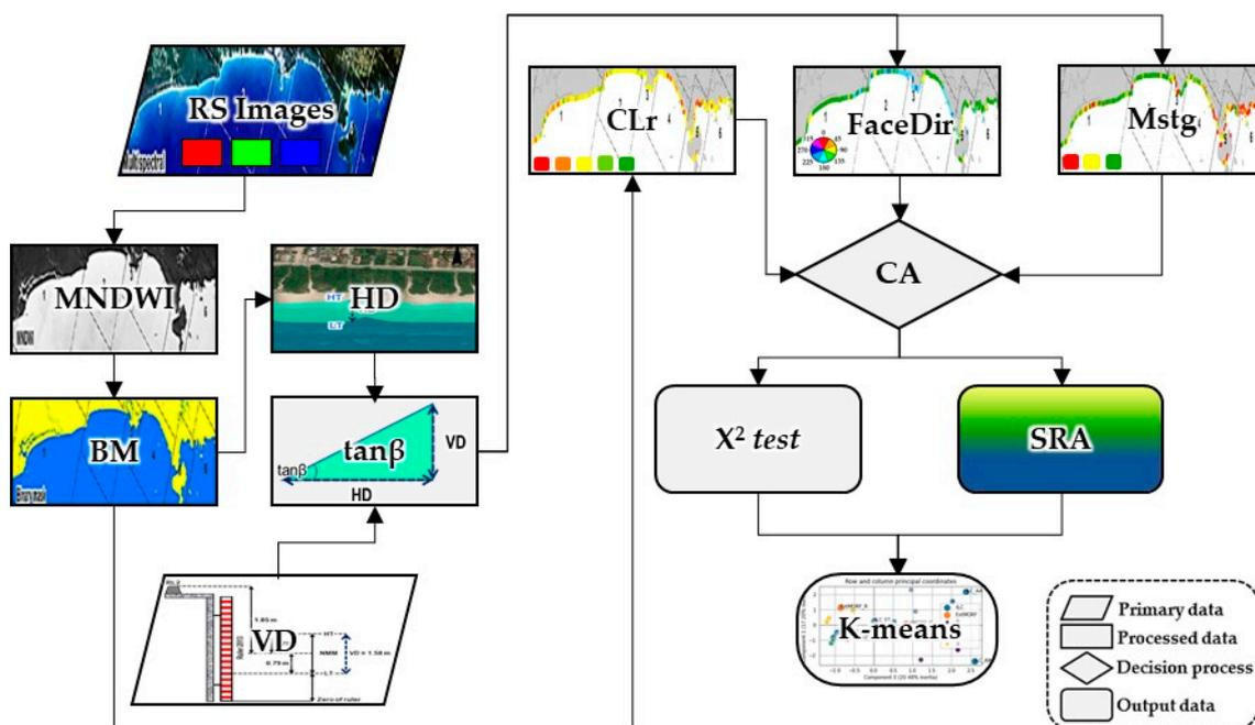
**Figure 2.** Flowchart of the steps in the methodology used in this research. RS: orbital remote sensing images; MNDWI: Modified normalized difference water index; BM: binary masks; HD: horizontal distance; VD: vertical distance;  $\tan\beta$ : slope; CLr: annual erosion and accretion rate; FaceDir: beach face direction; Mstg: morphodynamic stage trend; CA: correspondence analysis;  $X^2$ : chi-square test; SRA: standardized residual analysis; K-means: a cluster analysis.
