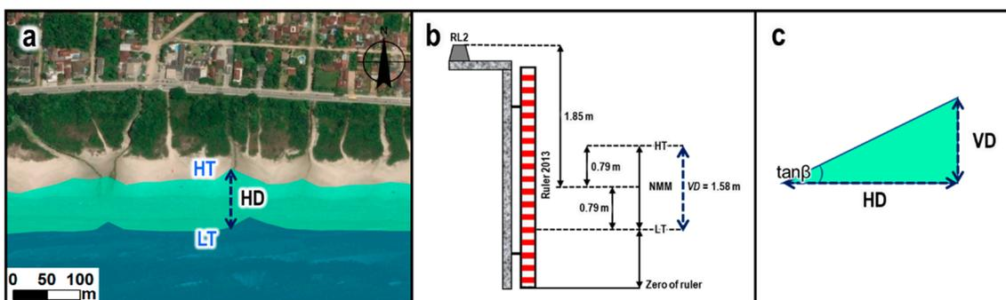
**Figure 4.** Shows three parameters: (a) the Horizontal Distance (HD) between the coastlines of Spring High Tide (HT) and Low Tide (LT), which was derived from satellite images; (b) The Vertical Distance (VD) of the tidal range near the port of Santos, São Paulo, Brazil [55,57] and (c) The slope ( $\tan\beta$ ) of the right triangle formed by the horizontal and vertical distances.
