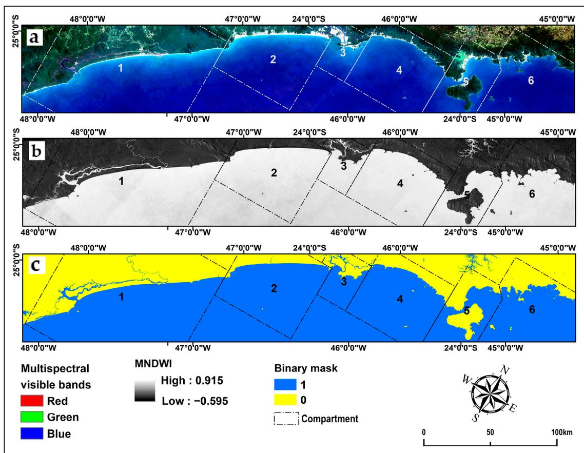
**Figure 3.** (a) Multispectral image of visible bands; (b) Modified Normalized Difference Water Index (MNDWI); (c) Binary mask with water classes “1” (blue) and land classes “0” (yellow), plus spatial mode filtering. Example from the average year of 2021 for the entire coastline of the State of São Paulo.
