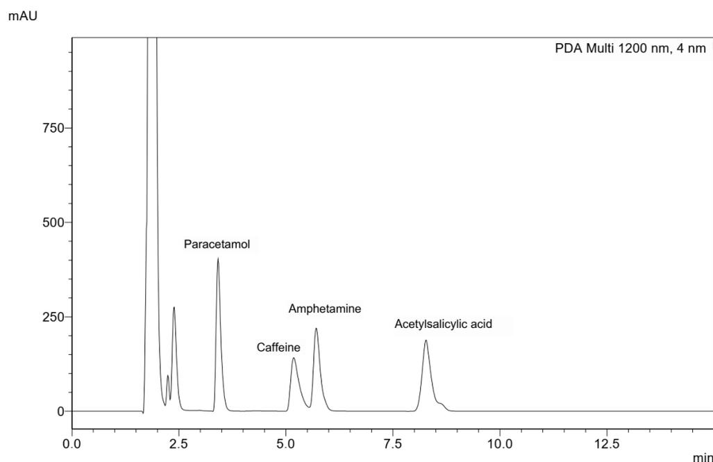
**Figure 3.** Separation of a mixture of amphetamine, caffeine, acetylsalicylic acid and paracetamol at concentrations of 10  $\mu\text{g}/\text{mL}$ .
