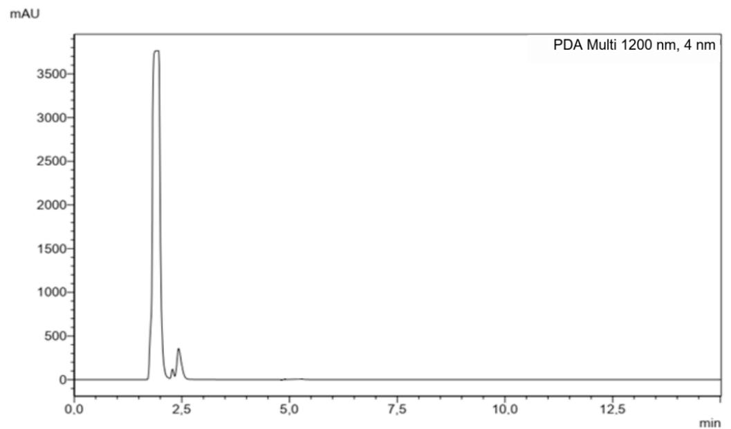
**Figure 1.** Chromatogram of synthetic urine diluent (amphetamine-free sample).
