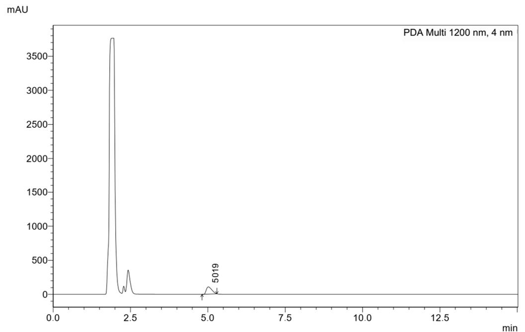
**Figure 2.** Chromatogram of a 10 µg/mL amphetamine solution in synthetic urine diluent.
