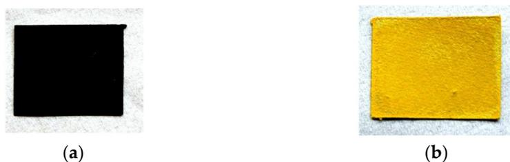
**Figure 26.** Color change response of the detection film: (a) the original black color of the unexposed film; (b) the yellow color of the film in presence of  $\text{NH}_3$  gas [7].
