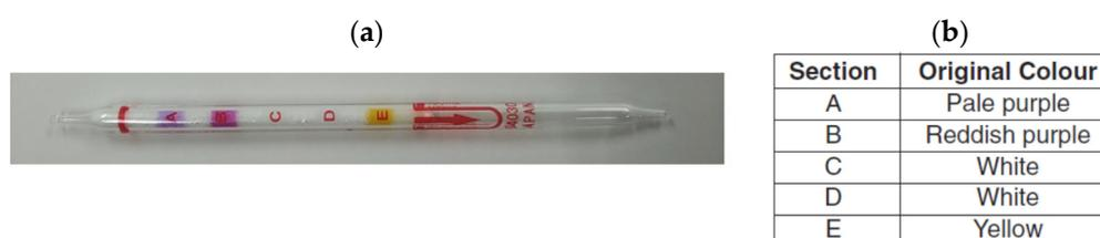
**Figure 12.** Inorganic gas qualitative detector tube: (a) picture of the detector tube; (b) original color. Adapted with permission from ref. [40]. Copyright 2021 Komyo Rikagaku Kogyo K.K.
