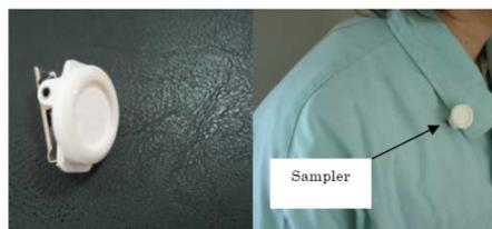
**Figure 25.** A passive sampling badge shown attached to a worker's collar for personal sampling and clipped in an appropriate location for use in a workplace. Adapted with permission from ref. [8] (pp. 59–83). Copyright 2004 Kawamura.
