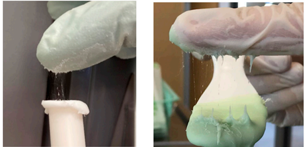
Figure 12. For low-viscosity cements, typical formation of threads on the glove (left Cemex System Genta; right Palacos LV hand-mixed).
