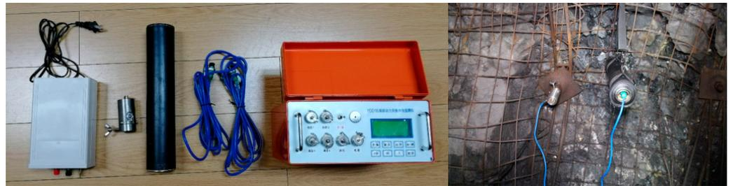
Figure 7. Portable coal and rock dynamic disaster acoustic and electrical monitor and field acoustic and electrical probe installation diagram.
