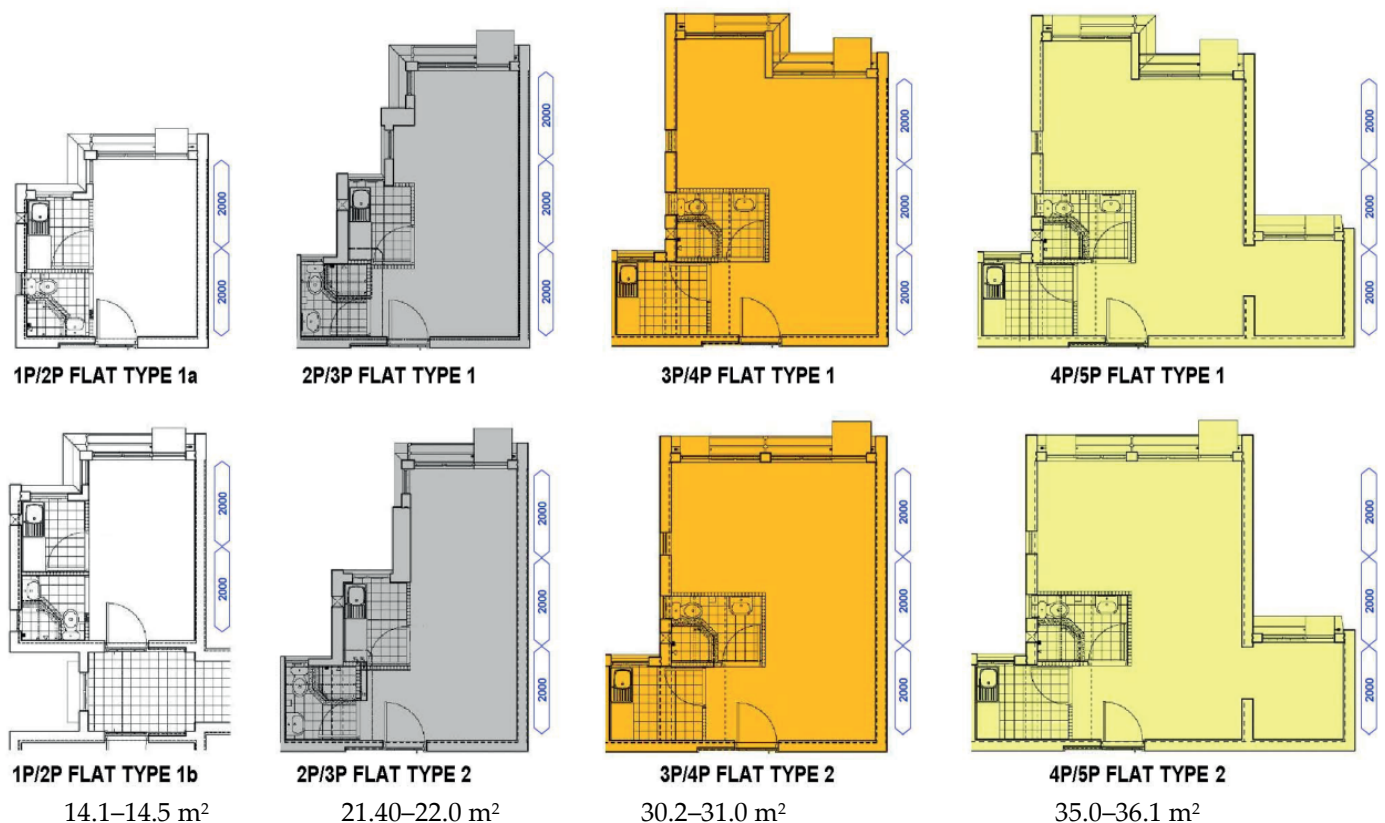
Figure 10. Modular flat design, 2013/2015 version. Source: Legislative Council Panel on Housing, Modular Flat Design for public housing development of the Hong Kong Housing Authority (2013) [49].
