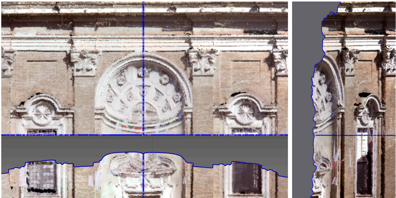
Figure 9. Elevation, plan, and section after the photographic model (elaboration of the author). In blue, the vertical and horizontal sections (image by M. Carpicci).
