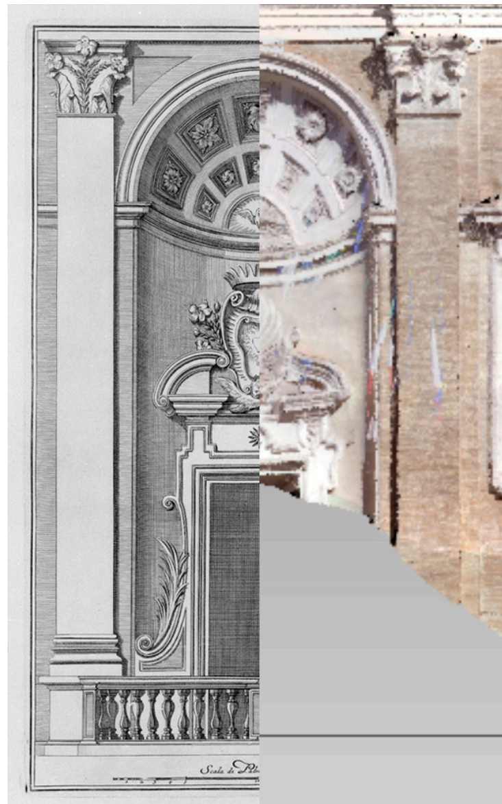
Figure 15. Comparison between Sebastiano Giannini's plate of the portal in the niche and the orthographic elevation after the photographic model (elaboration of the authors).
