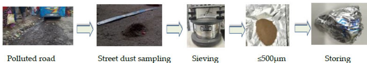
Figure 2. Road dust sample collection and preparation stage.
