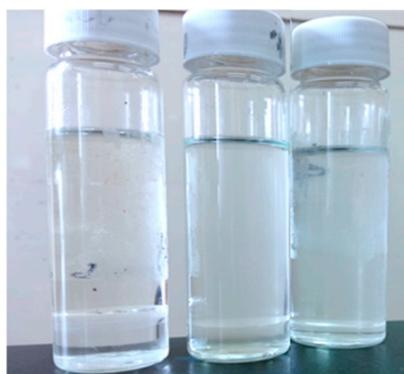
**Figure 3.** Biphasic system evaluated at the end of the esterification reaction of levulinic acid with 1-hexanol, carried out for 72 h, by using an alcohol: acid molar ratio equal to 1 and a catalyst loading equal to 1% (on the **right**), 5% (in the **middle**) and 10% (on the **left**) mol with respect to the acid.
