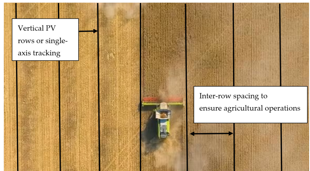
Figure 5. Agrivoltaic system pictorial design for wheat-growing agricultural land with sufficient spacing between solar PV rows ensuring ease of operation of agricultural machinery.
